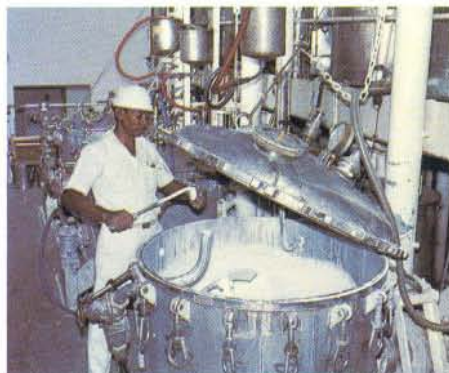
INDONESIA: Taking a sample of 'Pepsodent' toothpaste from one of the mixing vessels in our Surabaya factory.
